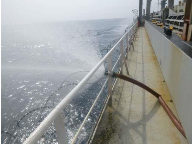
ACTIVATED FIRE HOSES AS PER BMP
