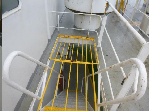
SECURITY GRATING INSTALLED AT STAIRCASE AS PART OF ANTI-PIRACY MEASURES
